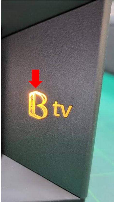
Poor Lasor cutting
